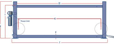
To calculate height constraints - measure floor to top of both vehicles add 12" to that figure.
