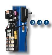
**B10264**: Air/electric workstation with filter/lubricator/regulator
